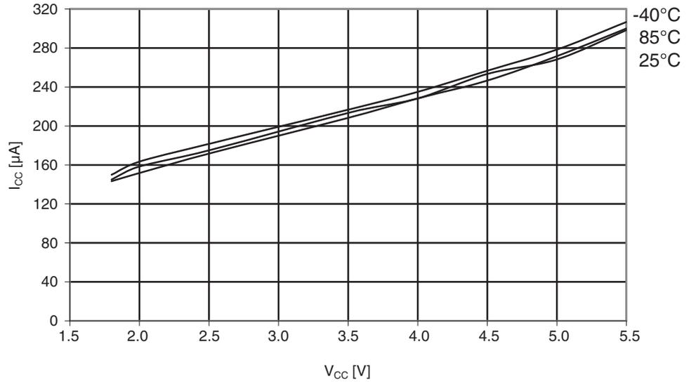
**Figure 29-91.** Atmel ATmega164PA: Analog comparator current vs.  $V_{CC}$ .
