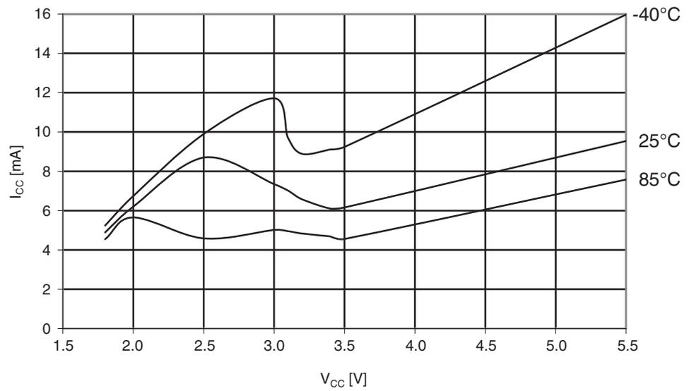
**Figure 29-242.** Atmel ATmega644A: Watchdog timer current vs.  $V_{CC}$ .
