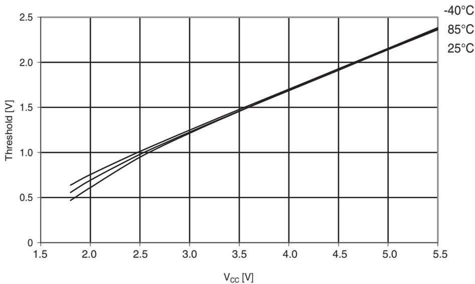
**Figure 29-125.**Atmel ATmega324A: I/O pin input hysteresis vs.  $V_{CC}$ .
