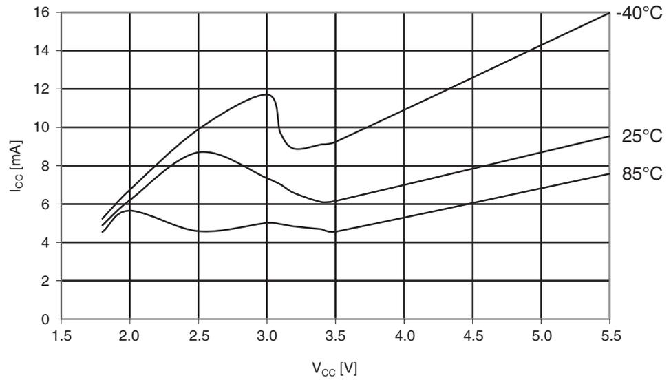
**Figure 29-291.**Atmel ATmega644PA: Watchdog timer current vs.  $V_{CC}$ .
