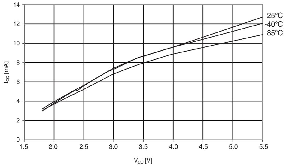
**Figure 29-193.**Atmel ATmega324PA: Watchdog timer current vs.  $V_{CC}$ .
