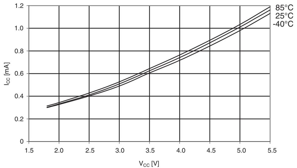
**Figure 29-54.** Atmel ATmega164PA: Active supply current vs.  $V_{CC}$  (internal RC oscillator, 128kHz).
