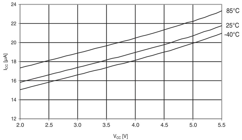
**Figure 29-241.** Atmel ATmega644A: Programming current vs.  $V_{CC}$ .
