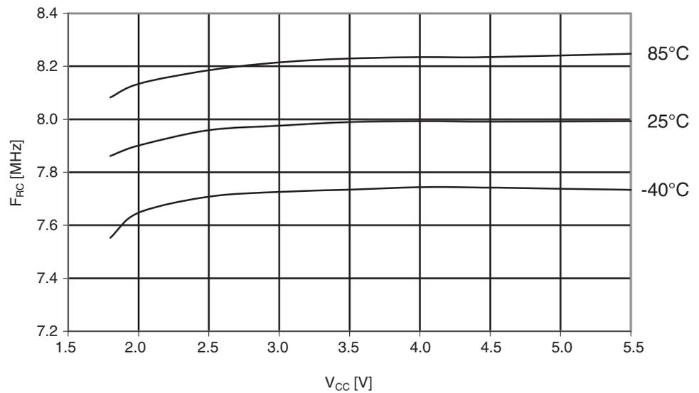
**Figure 29-39.** Atmel ATmega164A: Calibrated 8MHz RC oscillator vs. temperature.
