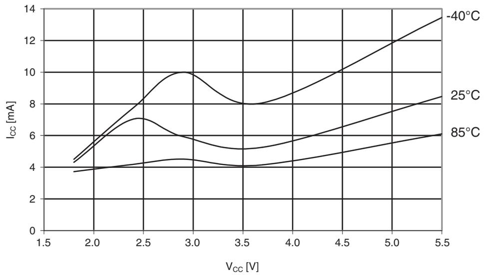
**Figure 29-391.**Atmel ATmega1284P: Watchdog timer current vs.  $V_{CC}$ .
