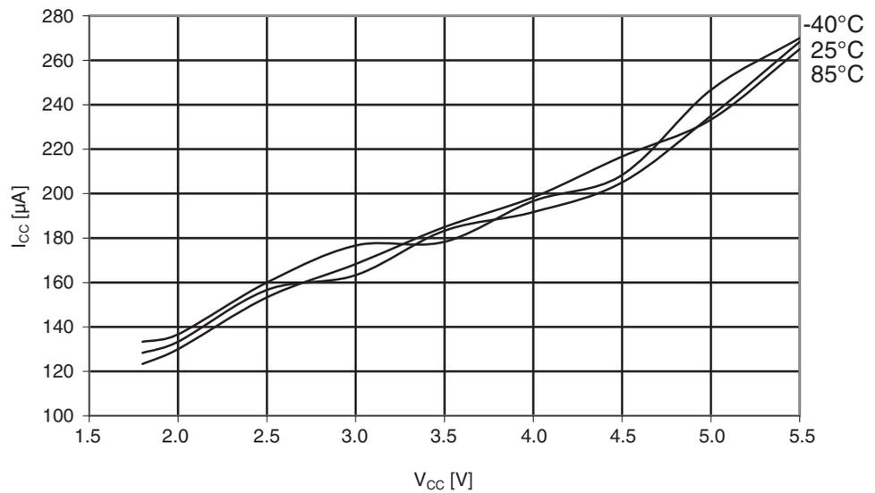
**Figure 29-337.**Atmel ATmega1284: Analog comparator current vs.  $V_{CC}$ .
