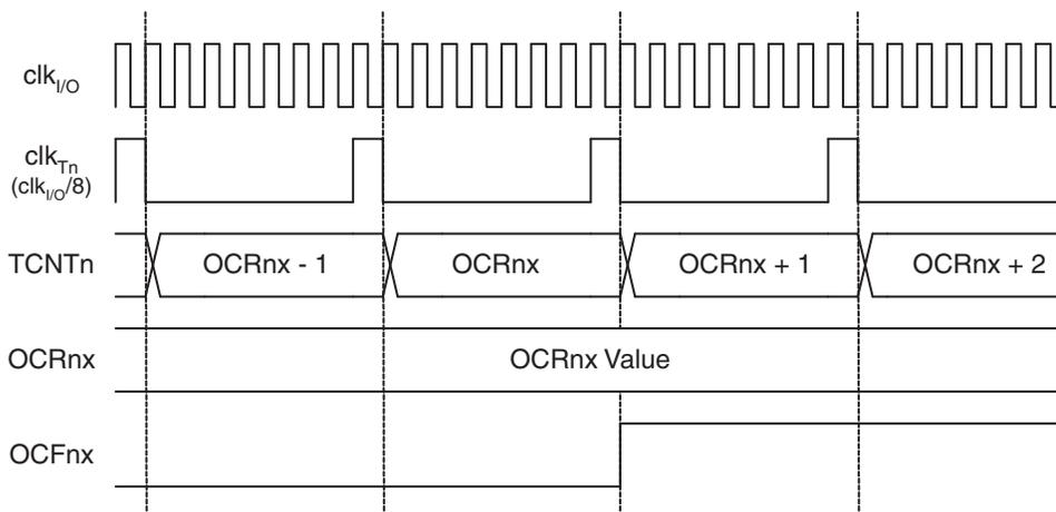
Figure 16-12 shows the count sequence close to TOP in various modes. When using phase and frequency correct PWM mode the OCRnx Register is updated at BOTTOM. The timing diagrams will be the same, but TOP should be replaced by BOTTOM, TOP-1 by BOTTOM+1 and so on. The same renaming applies for modes that set the TOVn Flag at BOTTOM.
