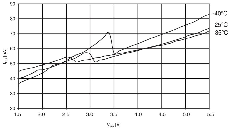
**Figure 29-239.**Atmel ATmega644A: AREF external reference current vs.  $V_{CC}$ .
