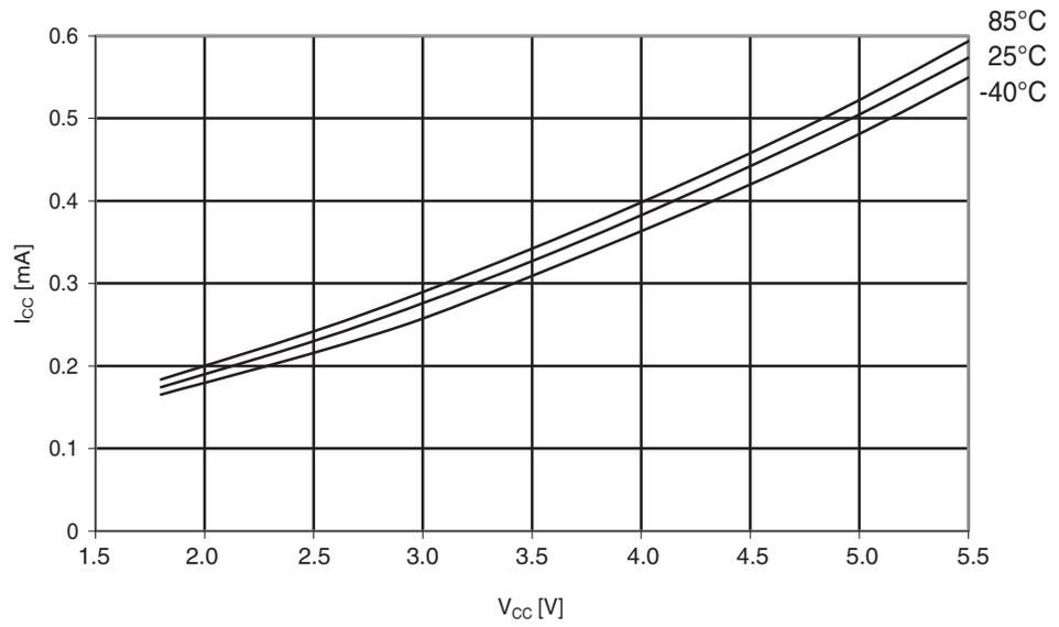
**Figure 29-157.**Atmel ATmega324PA: Idle supply current vs.  $V_{CC}$  (internal RC oscillator, 128kHz).
