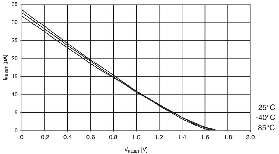
**Figure 29-264.** Atmel ATmega644PA: Reset pull-up resistor current vs. reset pin voltage ( $V_{CC} = 2.7V$ ).
