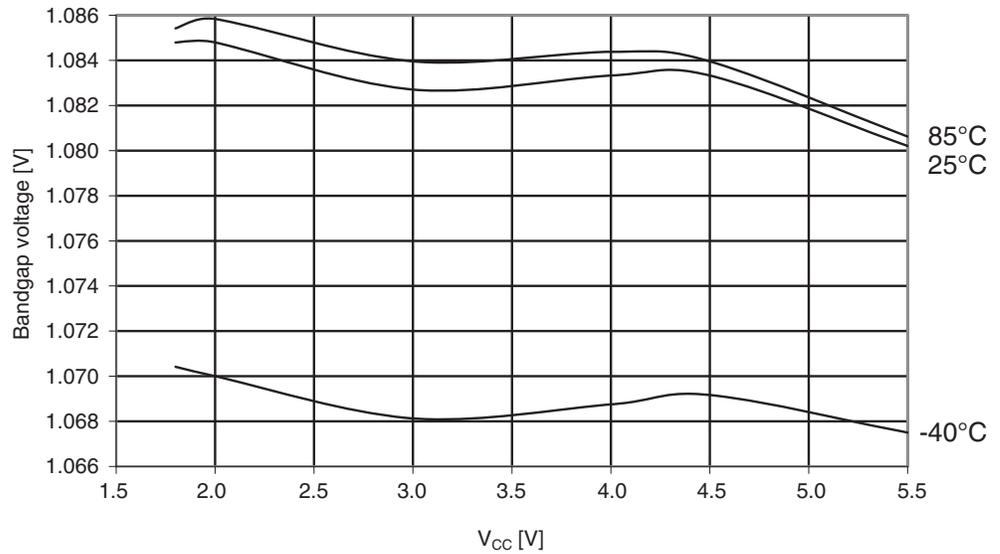
**Figure 29-231.**Atmel ATmega644A: Bandgap voltage vs. temperature.
