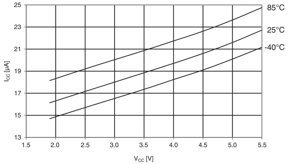
**Figure 29-340.**Atmel ATmega1284: Programming current vs.  $V_{CC}$ .
