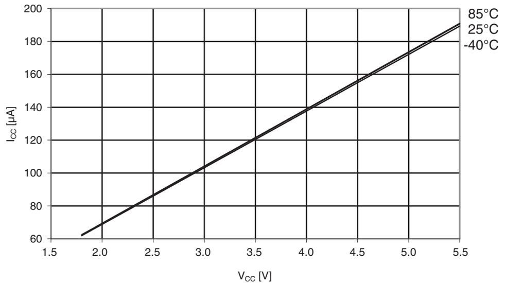
**Figure 29-339.**Atmel ATmega1284: Brownout detector current vs.  $V_{CC}$ .
