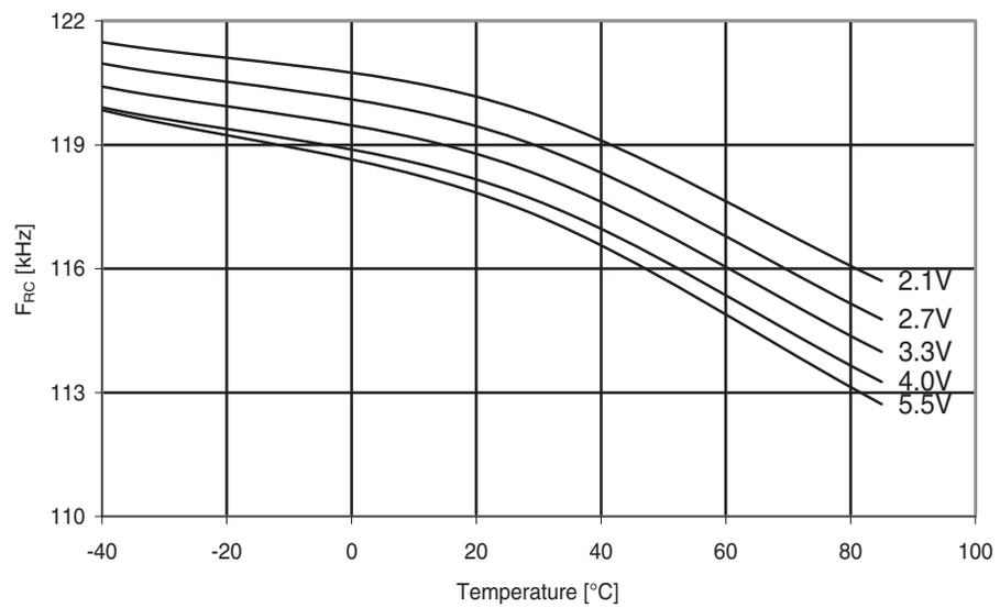
**Figure 29-135.**Atmel ATmega324A: Watchdog oscillator frequency vs.  $V_{CC}$ .
