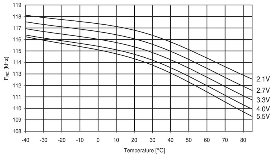
**Figure 29-233.**Atmel ATmega644A: Watchdog oscillator frequency vs.  $V_{CC}$ .
