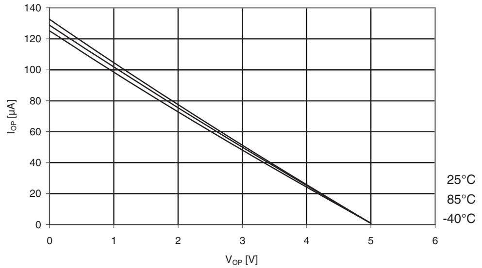
**Figure 29-67.** Atmel ATmega164PA: Reset pull-up resistor current vs. reset pin voltage ( $V_{CC} = 1.8V$ ).
