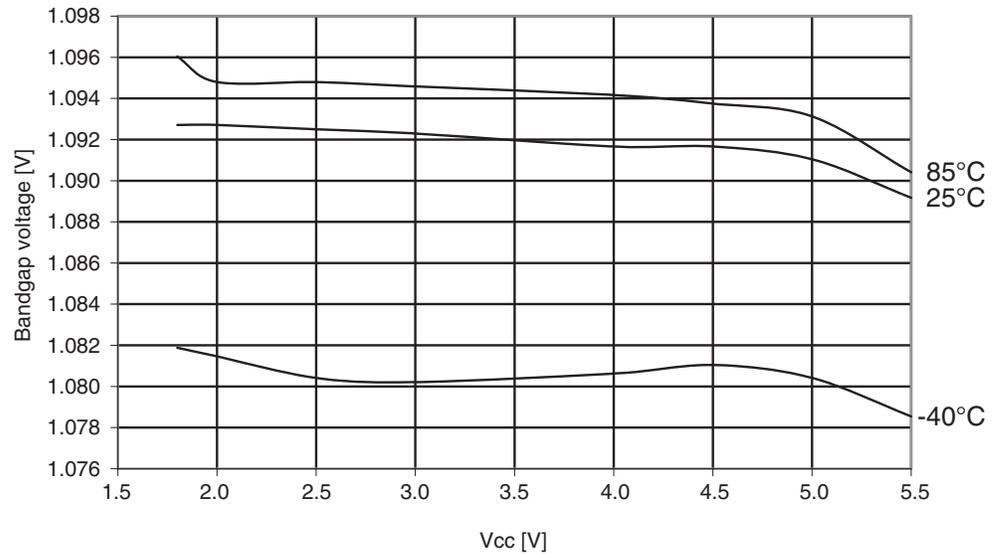
**Figure 29-182.**Atmel ATmega324PA: Bandgap voltage vs. temperature.
