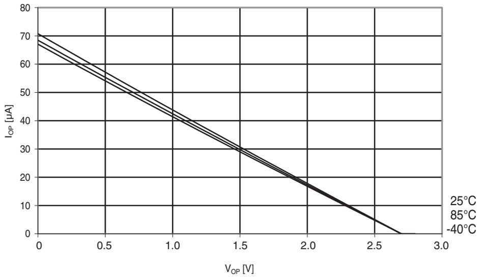
**Figure 29-262.** Atmel ATmega644PA: I/O pin pull-up resistor current vs. input voltage ( $V_{CC} = 5V$ ).
