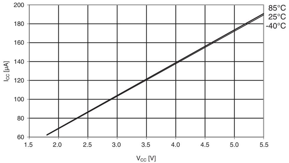
**Figure 29-389.**Atmel ATmega1284P: Brownout detector current vs.  $V_{CC}$ .
