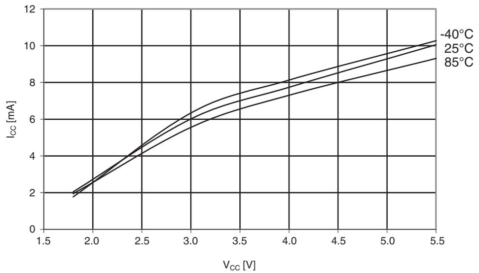
**Figure 29-46.** Atmel ATmega164A: Watchdog timer current vs.  $V_{CC}$ .
