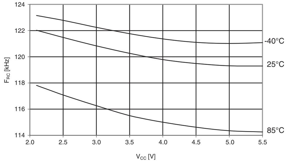
**Figure 29-383.**Atmel ATmega1284P: Calibrated 8MHz RC oscillator vs.  $V_{CC}$ .
