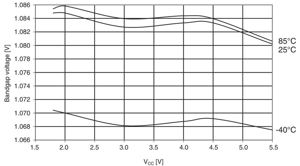
**Figure 29-280.**Atmel ATmega324PA: Bandgap voltage vs. temperature.
