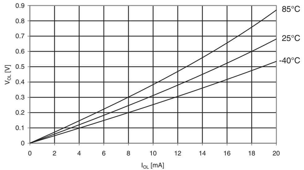
**Figure 29-367.** Atmel ATmega1284P: I/O pin output voltage vs. sink current ( $V_{CC} = 5V$ ).
