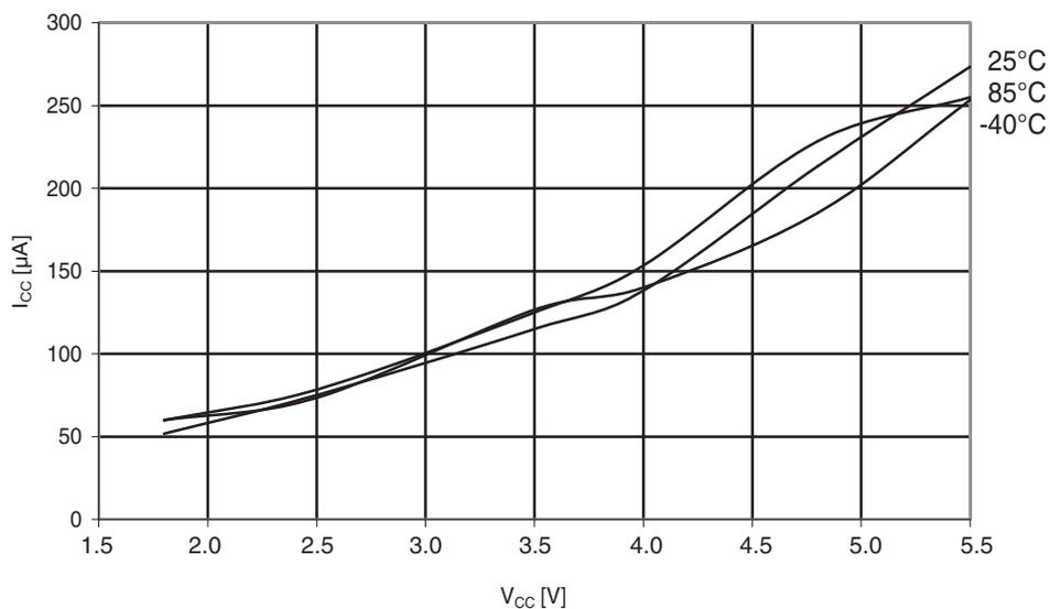
**Figure 29-189.**Atmel ATmega324PA: Analog comparator current vs.  $V_{CC}$ .
