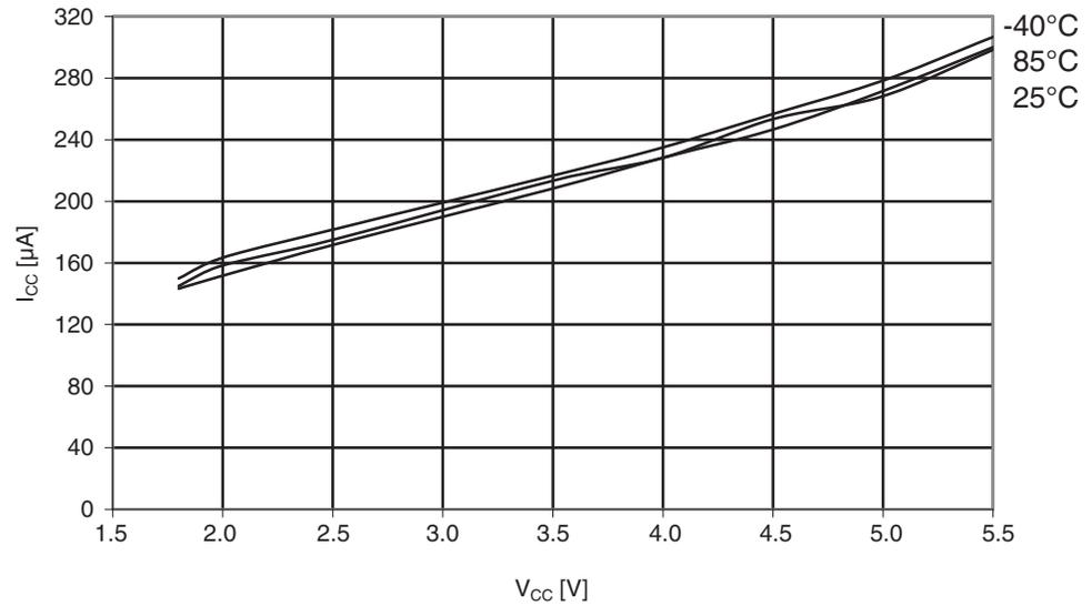
**Figure 29-42.** Atmel ATmega164A: Analog comparator current vs.  $V_{CC}$ .
