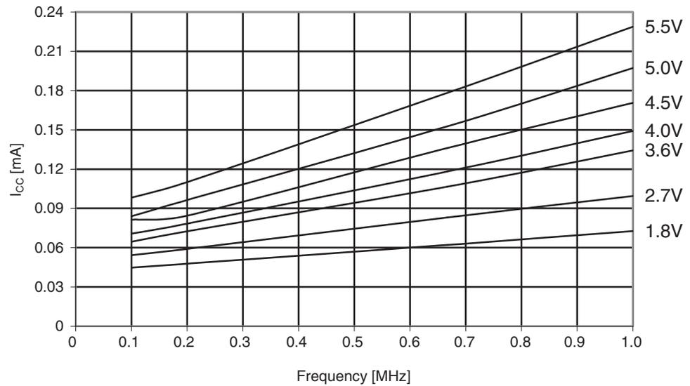
**Figure 29-351.** Atmel ATmega1284P: Idle supply current vs. frequency (1 - 20MHz).
