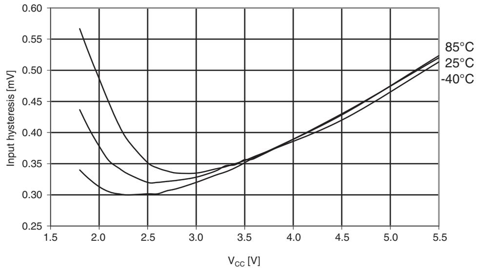
**Figure 29-323.** Atmel ATmega1284: Reset pin input threshold vs.  $V_{CC}$  ( $V_{IH}$ , I/O pin read as '1').
