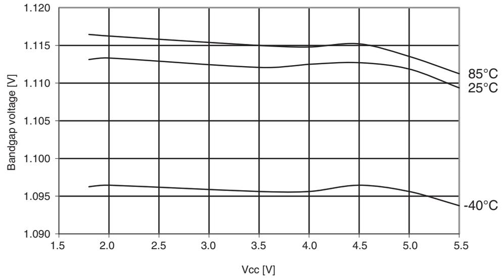
**Figure 29-380.**Atmel ATmega1284P: Bandgap voltage vs. temperature.
