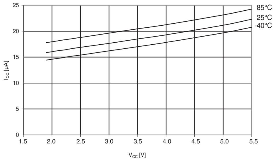
**Figure 29-192.**Atmel ATmega324PA: Programming current vs.  $V_{CC}$ .
