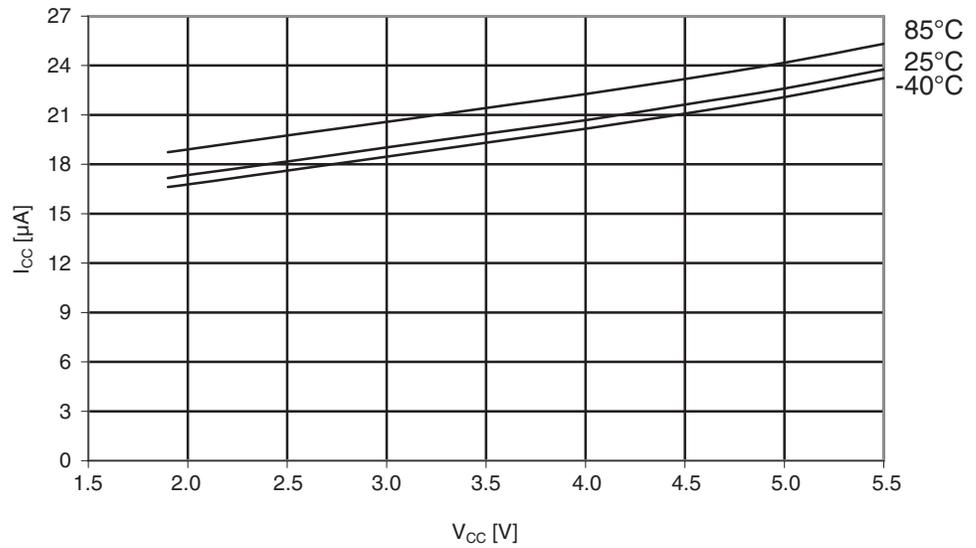
**Figure 29-45.** Atmel ATmega164A: Programming current vs.  $V_{CC}$ .
