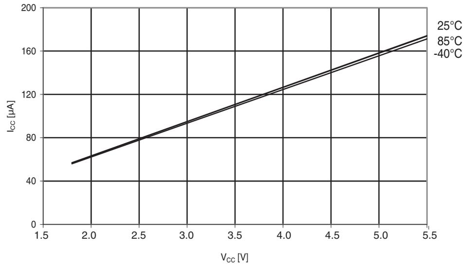
**Figure 29-240.**Atmel ATmega644A: Brownout detector current vs.  $V_{CC}$ .
