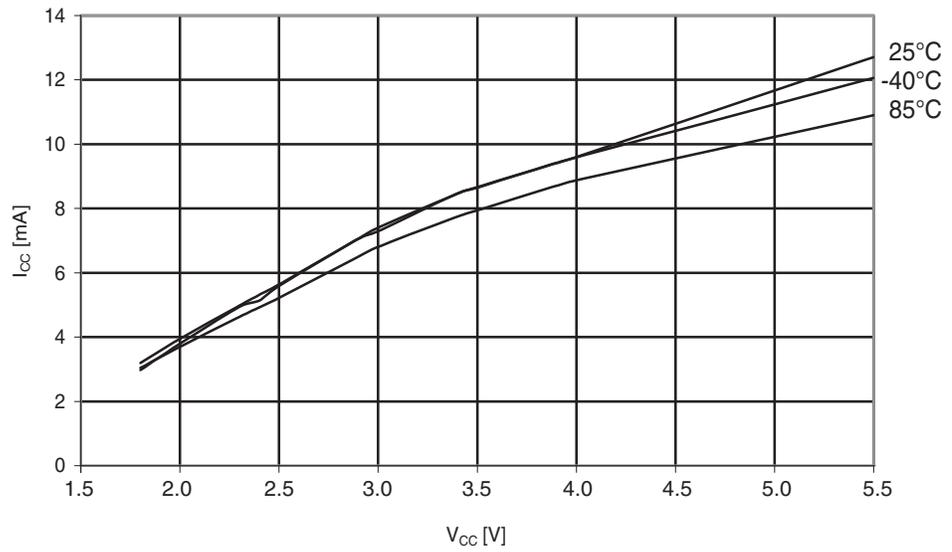
**Figure 29-144.** Atmel ATmega324A: Watchdog timer current vs.  $V_{CC}$ .
