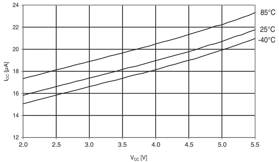
**Figure 29-290.**Atmel ATmega644PA: Programming current vs.  $V_{CC}$ .
