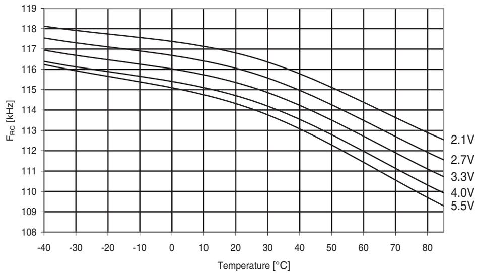
**Figure 29-282.**Atmel ATmega644PA: Watchdog oscillator frequency vs.  $V_{CC}$ .
