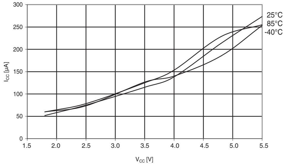
**Figure 29-140.** Atmel ATmega324A: Analog comparator current vs.  $V_{CC}$ .
