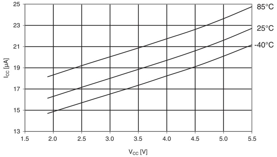
**Figure 29-390.**Atmel ATmega1284P: Programming current vs.  $V_{CC}$ .
