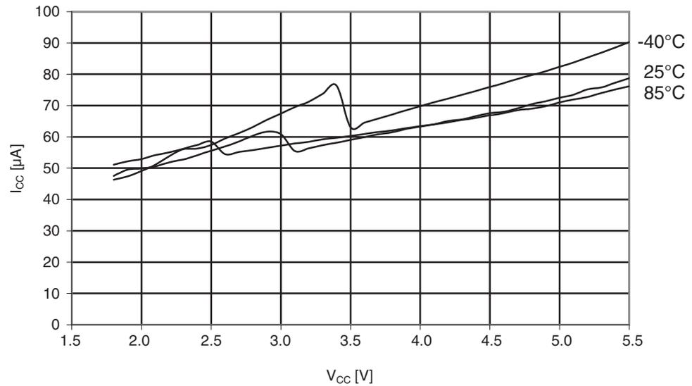
**Figure 29-43.** Atmel ATmega164A: AREF external reference current vs.  $V_{CC}$ .
