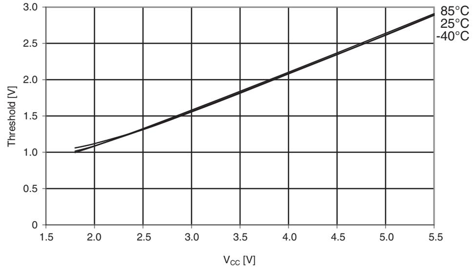
**Figure 29-371.** Atmel ATmega1284P: I/O pin input threshold vs.  $V_{CC}$  ( $V_{IL}$ , I/O pin read as '0').
