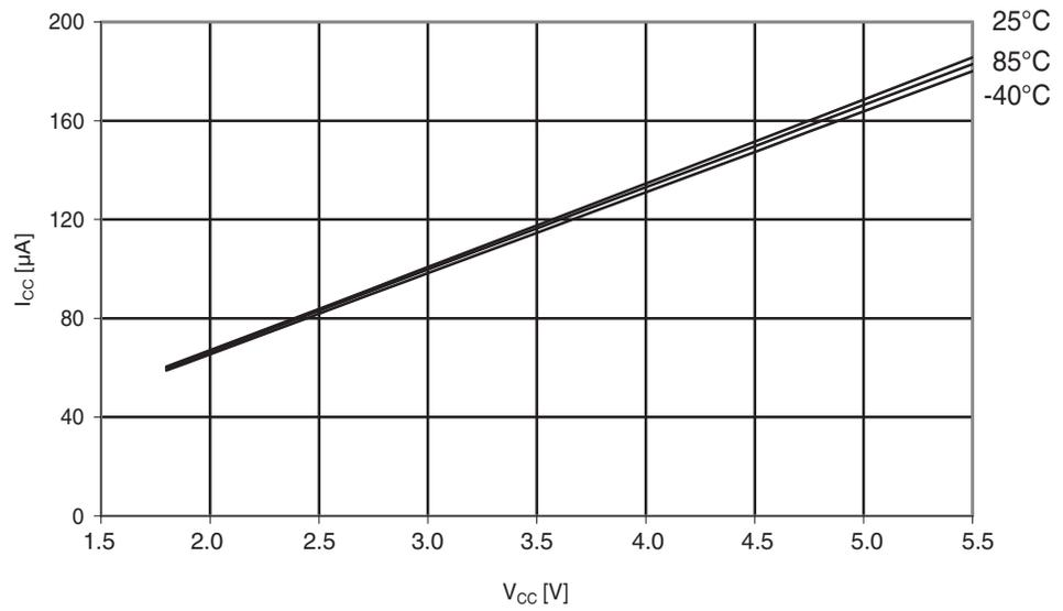
**Figure 29-191.**Atmel ATmega324PA: Brownout detector current vs.  $V_{CC}$ .
