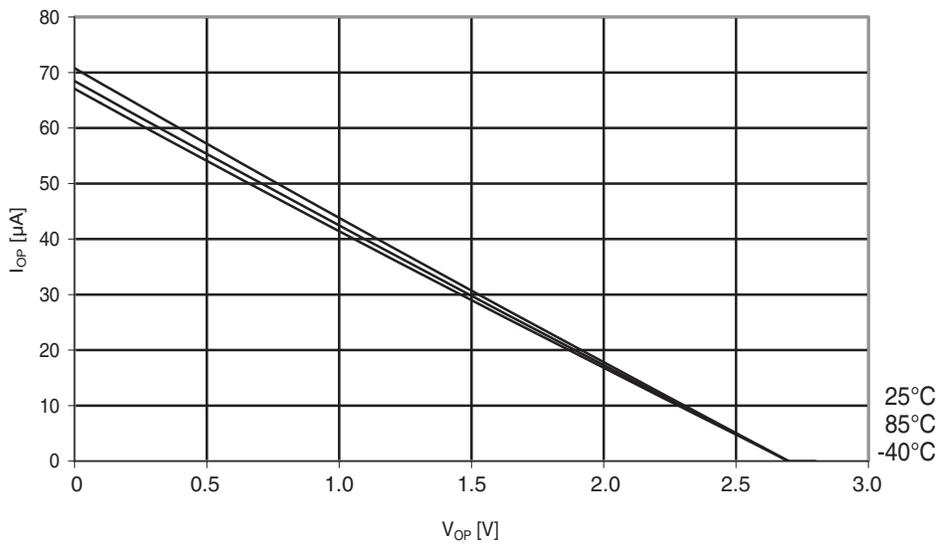
**Figure 29-213.** Atmel ATmega644A: I/O pin pull-up resistor current vs. input voltage ( $V_{CC} = 5V$ ).
