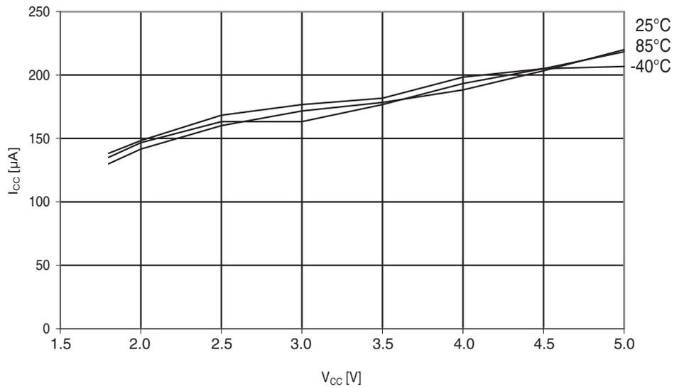
**Figure 29-238.** Atmel ATmega644A: Analog comparator current vs.  $V_{CC}$ .
