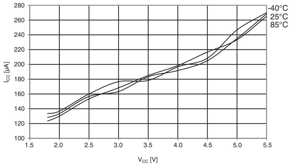
**Figure 29-387.**Atmel ATmega1284P: Analog comparator current vs.  $V_{CC}$ .
