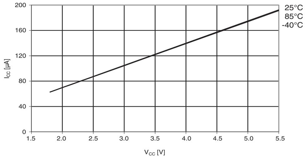
**Figure 29-44.** Atmel ATmega164A: Brownout detector current vs.  $V_{CC}$ .
