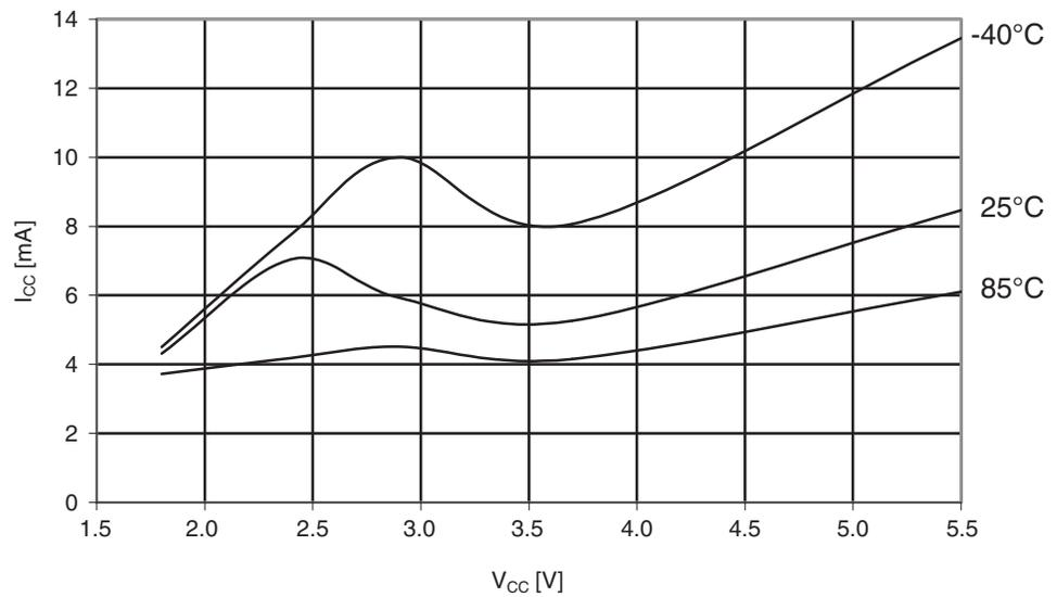
**Figure 29-341.** Atmel ATmega1284: Watchdog timer current vs.  $V_{CC}$ .
