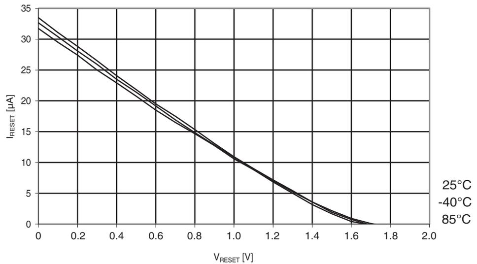
**Figure 29-215.** Atmel ATmega644A: Reset pull-up resistor current vs. reset pin voltage ( $V_{CC} = 2.7V$ ).
