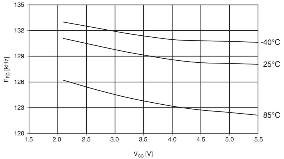
**Figure 29-87.** Atmel ATmega164PA: Calibrated 8MHz RC oscillator vs.  $V_{CC}$ .
