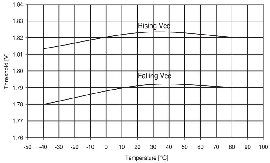
**Figure 29-230.** Atmel ATmega644A: Calibrated bandgap voltage vs.  $V_{CC}$ .
