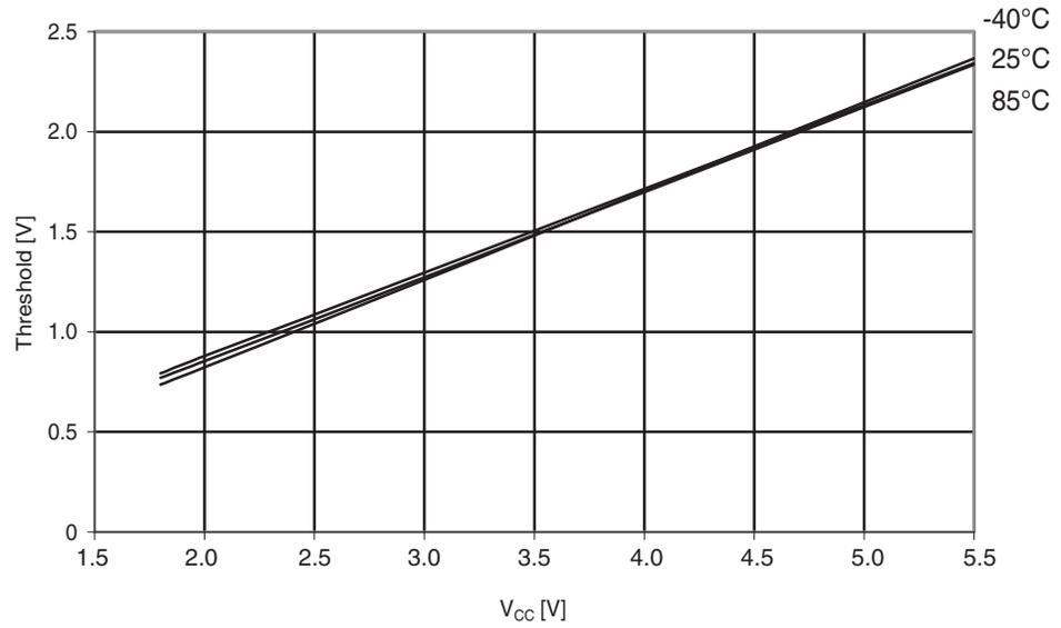
**Figure 29-177.** Atmel ATmega324PA: Reset pin input hysteresis vs.  $V_{CC}$ .
