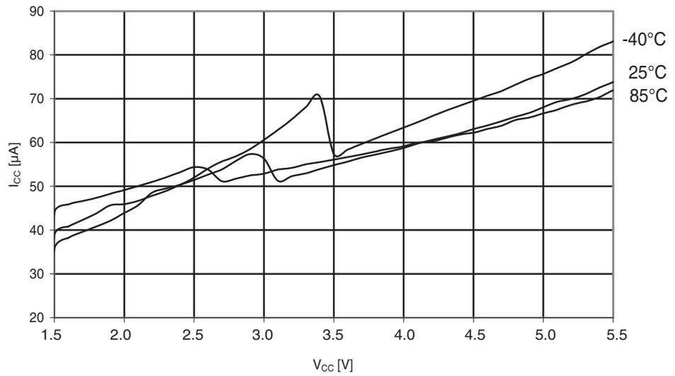
**Figure 29-288.**Atmel ATmega644PA: AREF external reference current vs.  $V_{CC}$ .
