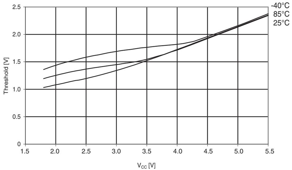
**Figure 29-176.** Atmel ATmega324PA: Reset pin input threshold vs.  $V_{CC}$  ( $V_{IL}$ , I/O pin read as '0').
