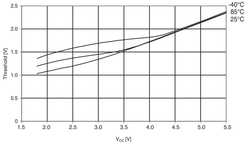
**Figure 29-127.** Atmel ATmega324A: Reset pin input threshold vs.  $V_{CC}$  ( $V_{IL}$ , I/O pin read as '0').
