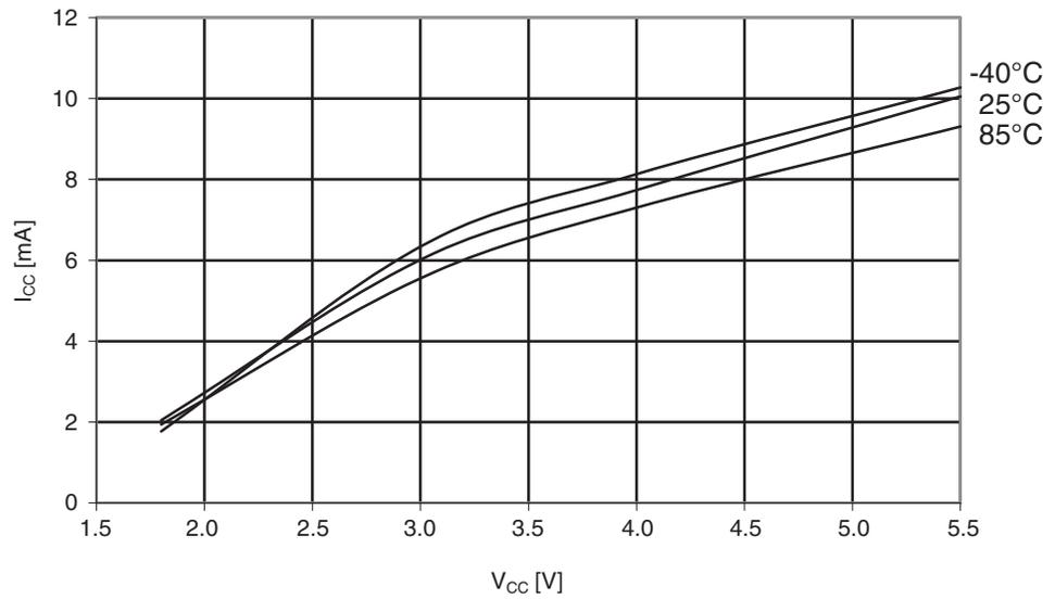
**Figure 29-95.** Atmel ATmega164PA: Watchdog timer current vs.  $V_{CC}$ .
