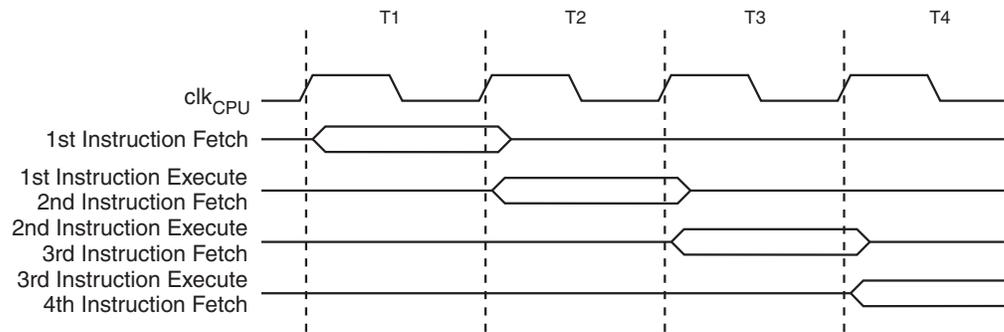
Figure 7-6 shows the internal timing concept for the Register File. In a single clock cycle an ALU operation using two register operands is executed, and the result is stored back to the destination register.
