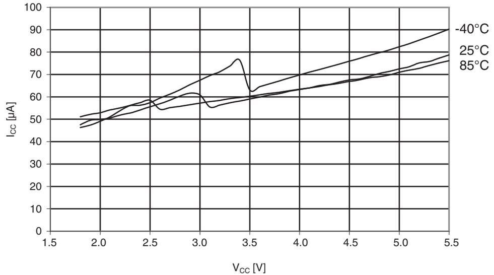
**Figure 29-92.** Atmel ATmega164PA: AREF external reference current vs.  $V_{CC}$ .
