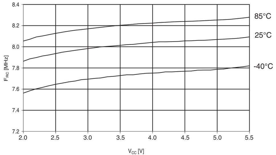
**Figure 29-284.**Atmel ATmega644PA: Calibrated 8MHz RC oscillator vs. temperature.
