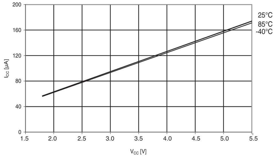
**Figure 29-289.**Atmel ATmega644PA: Brownout detector current vs.  $V_{CC}$ .
